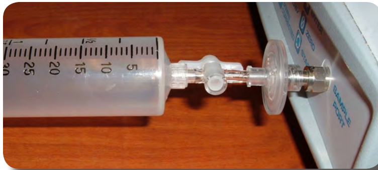
Inject Full Calibration Gas
