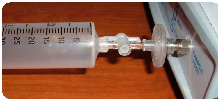
Inject Full Calibration Gas
