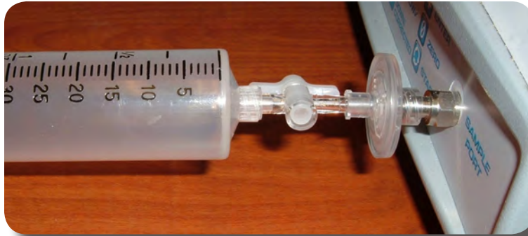
Inject Full Calibration Gas
